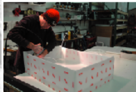
Screenprint equipment fabricator Taylor Ashcraft welds up a KDL KnockDown sink.
