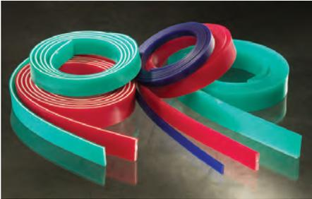
**serilor®SR** squeegee is an all purpose polyurethane blade with good combined resistance to chemicals and abrasion. It was developed to withstand various applications in screen printing. The industry standard S1 is a universal grade, your ideal choice for non critical abrasive application or when using common screen inks.
