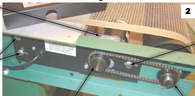
**Control assembly mounting screw (3 total)**
