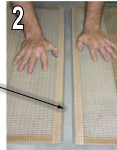
3) The belt needs to be tightened and adjusted. To tighten and adjust the belt, use the Aligner Bolts. To raise the Aligner, turn the Aligner Bolt clockwise with a 7/16" wrench. To lower it, turn it counter clockwise. Raise the Aligner until you have about 2"-2½" of slack as shown on right. Additional details on PAGE 7.
