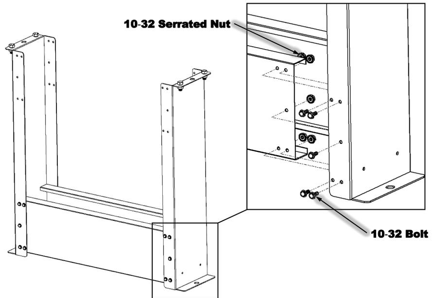
**1b)** Each conveyor has a pair of legs, a Front section, Rear Section, and middle conveyor pieces. Bolt together each section, as shown in the diagrams. Refer to **Page 18** for each conveyor's specific layout.
